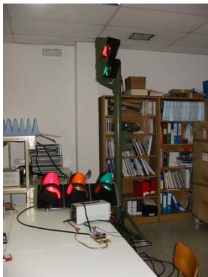
Figure 9. Testbed for the smart traffic light control based on PLC.
